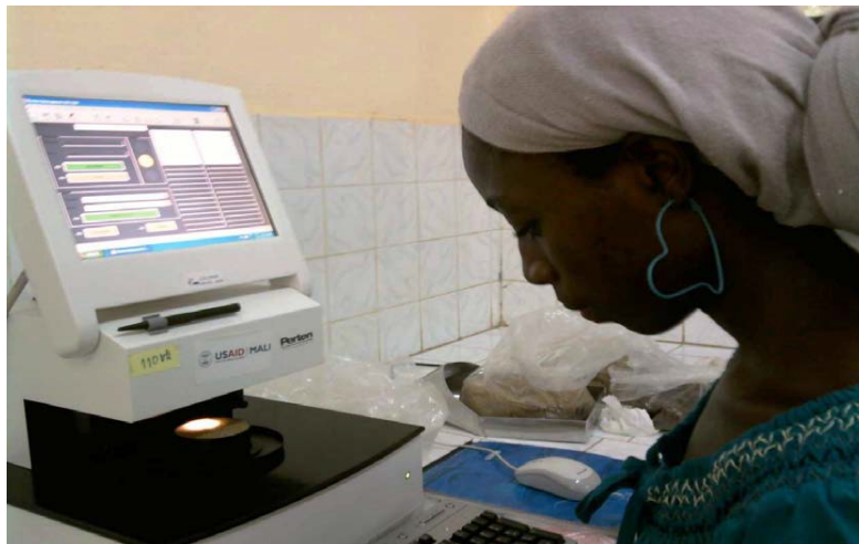
Figure 10. IPR student scanning samples with bench top Perten NIRS instrument at the IPR laboratory in Katibougou.
